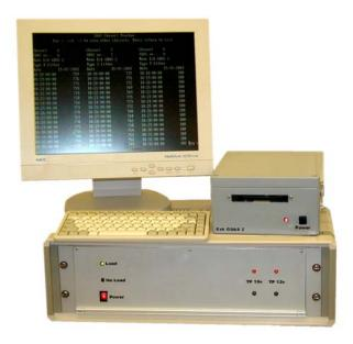
To prevent loss of data due to interruptions in the mains supply the complete system operates from a single 12 volt battery which gives several hours autonomy in the event of failure of the mains supply.
