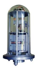
Total field (F) data are derived from a GEM Systems, GSM-90 Overhauser magnetometer in situ at Eskdalemuir. The GSM-90 has 0.01 nT resolution, 0.2 nT absolute accuracy and long-term stability of 0.05 nT / year. Dynamic range is from 20,000 to 120,000 nT.
